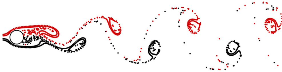
Fig. 9. Massless particle flow behind a circular cylinder at Re = 100 in the developed flow stage; t = 200 .
