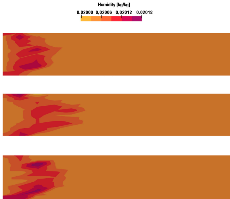
Fig. 6. Humidity field inside the drying chamber at three different cross section planes (see Fig. 1) after drying time of 0.15 s.
